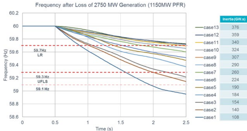
Figure 8: Frequency Response after loss of 2,750 MW for 13 cases with different inertia levels
